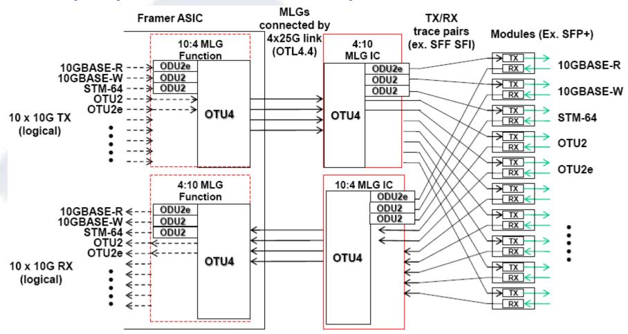
OTN mapping enables heterogeneous combination of 10G port types with independent timing (except -KR)
